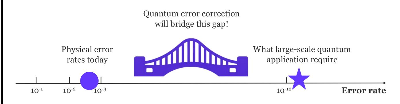
QEC is expensive: to factor a 2048-bit integer, we need thousands of noise-resilient qubits, which cost us million(s) of noisy qubits to simulate. How can we reduce this daunting cost and build efficient, scalable quantum computers for the future?
