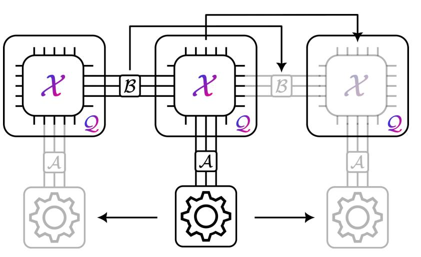
In a mobile neutral atom array, the many components of an extractor architecture can all be mobile.
